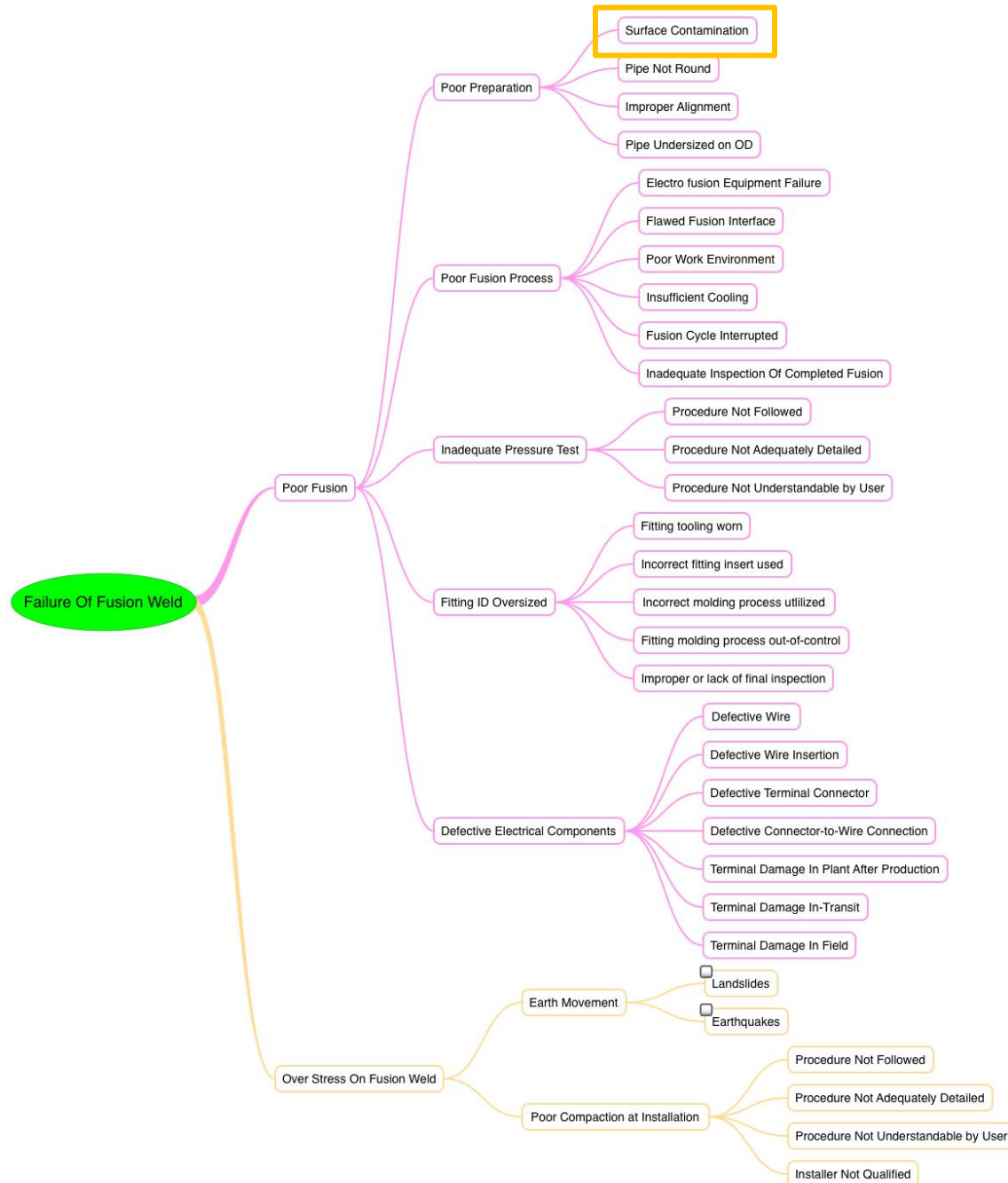
Figure 2: High-Level Fault Tree for Contaminated Electrofusion Weld
