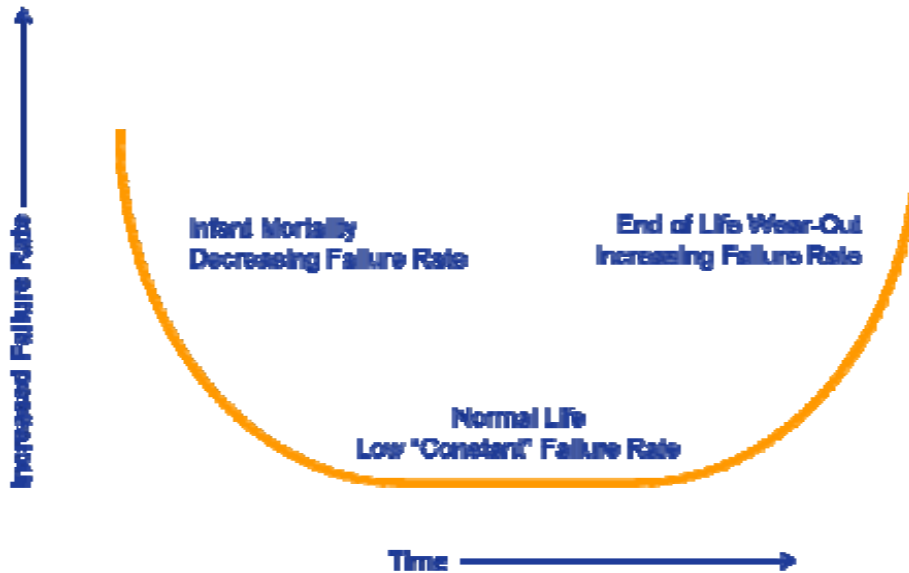
Figure 2: Typical Product Bathtub Failure Rate Curve
