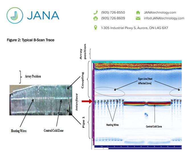
The B-Scan output appears as a picture of a section through the weld, with the reflections from the heating wires, material interfaces and other reflection points identified. The B-Scan technique is typically 10-20 times more expensive than the single probe, much larger to handle and requires an expert to interpret the results.
