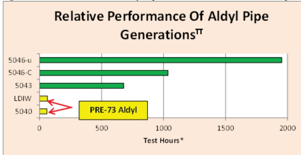
Note: <sup>a</sup>Based on testing at single condition. For more detailed performance characterizations see section on Performance Comparison of Aldyl Materials. \*Testing conducted at 80°C on 2" Pipe at nominal test stresses of 450-470 psi with Water internal/Water external. All failures were SCG failures initiating at the inner pipe bore.
