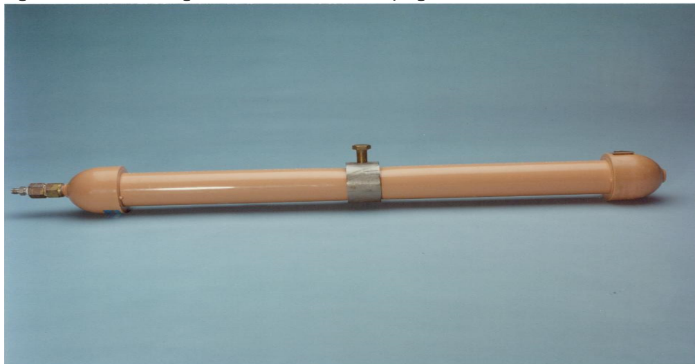
Figure 2: Indentation Jig for Simulation of Rock Impingement
